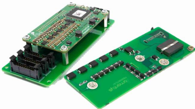
4500V Gate Drive example with Isolated DC DC Converter
