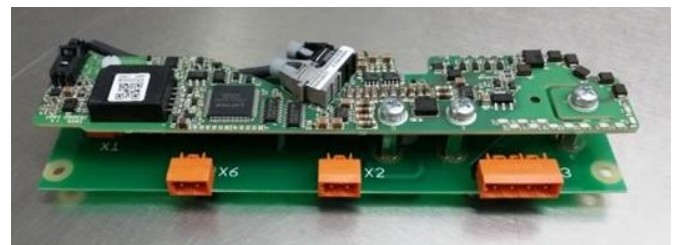
Figure [3] – Amantys Gate Drive Adapted for legacy traction converter
