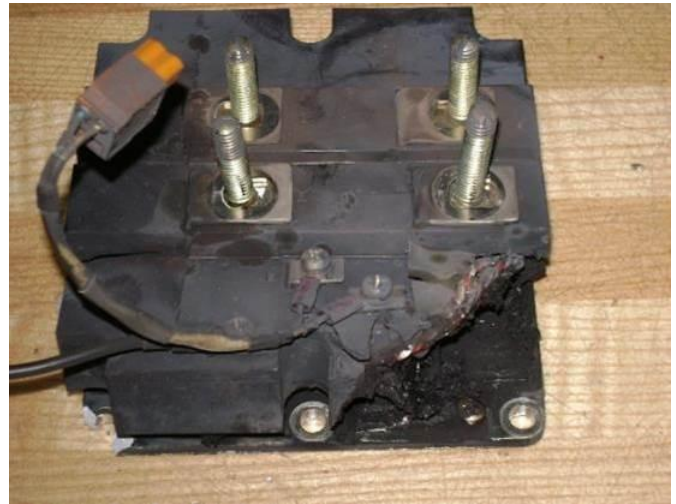
Figure [1] – Example of a failed IGBT
