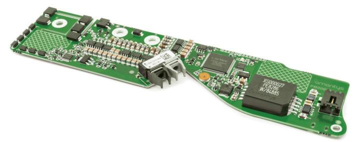
The Amantys 3300V Gate Drive will drive 3300V IGBT modules for 2-level and multi-level applications. The gate drive incorporates protection features for the IGBT module and can be configured by the user to optimise the operation of the gate drive in the power stack of the end application. 1200V and 1700V variants are also available.
