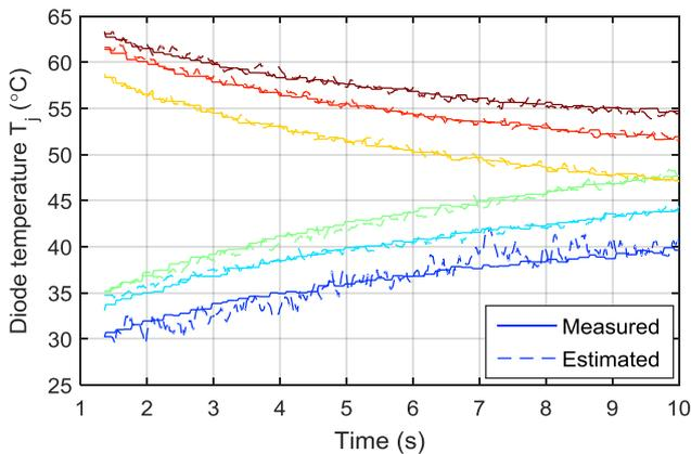
Matching of diode junction temperature estimate for both heating and cooling mission profiles.
