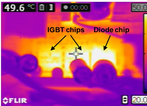
Chip temperature measurement with IR camera.
