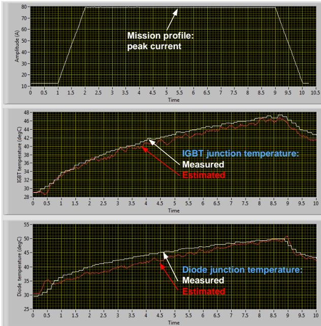
Matching of junction temperature estimation with temperatures measured by IR sensors.
